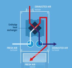
With the dedicated kit, a double-flow HRV unit with heat recovery can be integrated with the Unico Vertical-NK. In addition to the traditional functions of heating and cooling, it can also ensure an efficient and effective air exchange, thus improving indoor air quality and system efficiency.
